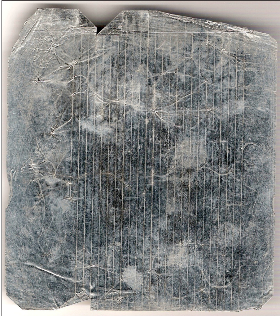
Fig. 1: Tinfoil fragment with twenty-four grooves, produced on Edison phonograph (c. 1877).
